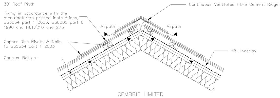
INSULATION AT RAFTER LEVEL (WARM ROOF)
